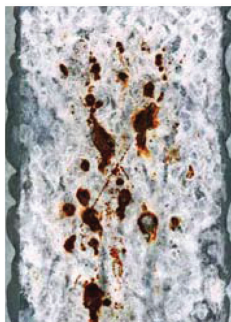
Galvanised steel Z275 @ 240 hours of salt spray testing.
